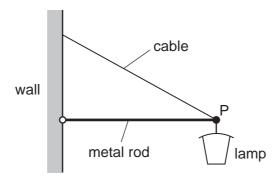
Which vector triangle could represent the forces acting on the end of the rod at point P?
