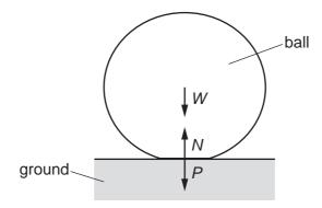
When the ball is in contact with the ground, the ball is momentarily stationary.
