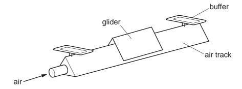
At each end of the air track, the glider has a perfectly elastic collision with a fixed buffer.
